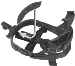
FIGURE 6-1. REMOVAL AND INSTALLATION OF BROWPAD
