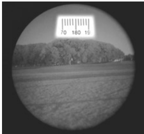
Figure 2-12. View Through Installed Compass
