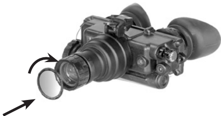
Figure 2-5. Installation of the Light Interference Filter
